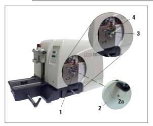
The feather key (4) is loosely placed in the handwheel shaft (1) and fixed in place with a tie-rap during transport.
