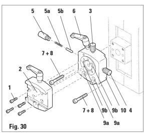
Finally, place the dovetail holder (2) and fasten by screwing in the 4 screws (1) using an Allen key size 3.
