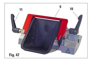
Knife holder E with water bath is available for both low profile, and high profile, blades.
