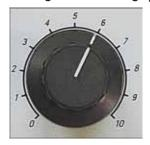
The sectioning speed can be set continuously (in the range of 0 - 420 mm/s) using the rotary knob.
