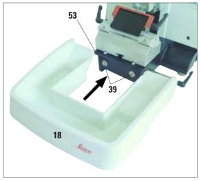
is held in place by the two magnets (39) (on the front of the microtome base plate). To remove the section waste tray, lift it slightly and pull it off towards the back.
