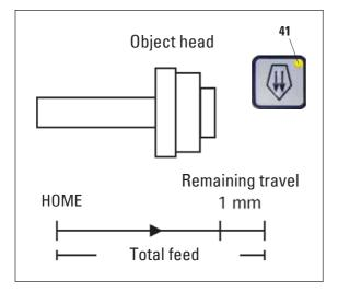
The visible and audible remaining feed indication feature informs the user during trimming and sectioning when a remaining feed of approximately 1 mm is available before the front limit is reached.
